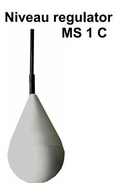
The Niveau regulator MS 1 C is a single point controller that is especially designed for use in extreme applications. It has a very high chemical resistance and is suitable for use in temperatures up to 100° C. The switch has gold platted contacts and can operate in circuits with a low switching current.
